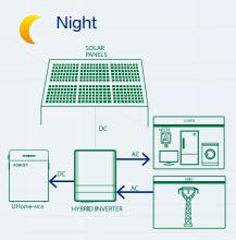
If the battery capacity is insufficient to meet selfconsumption requirement, electricity will be obtained from the grid.
