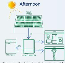
Extra energy will be fed into the grid when batteries are fully charged and system has already met its selfconsumption requirement.
