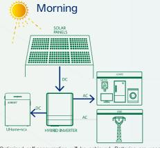
Optimized self-consumption will be achieved. Batteries are used to store the excess energy produced by PV System.
